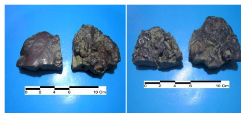
Fig8. Right: Upper Surface of the Flat Slags with Flow Wrinkles; Left: Lower Surface of the Specimen with Flat Morphology at the Left in Contrast to Irregular Morphology of Upper Surface at the Right.
