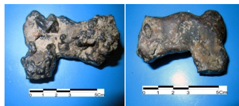
Fig10. Right: Upper Surface of the Specimen with Bulging, Reform Morphology that Reflects Plastic Deformations of the Melt during its Freezing Process; Left: Lower Surface of the Specimen Characterized by Relatively Irregular Morphology, Concentration of Secondary White Minerals Around
