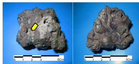
Fig9. Right: Upper Surface of the Branching Slag with Semi-Cylindrical Section; Left: Lower Surface of the Specimen with Irregular Morphology as a Function of the Irregularity of the Ground Surface. The Shape of the Slag Probably Followed the Shape of the Channel that Directed the Smelt From the Furnace into the Separation Pit Wherein Iron Was Separated From Silicate Melt.
