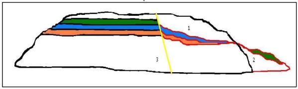
**Fig. 6** Schematic Design of Landslides Occurrence Mechanism,1: Empty Zone,2: Accumulation of Displaced Material, 3: Boundary Level of Rupture.
