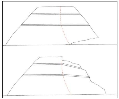
**Fig. 5** Schematic Design of Landslides Occurrence Mechanism, Water Permeation on Southern Slopes of Tepe
