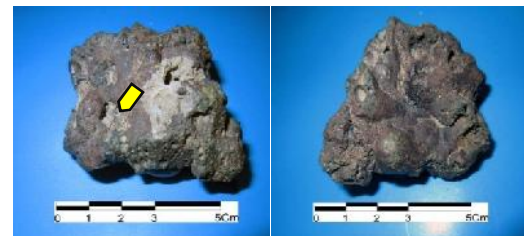
Fig9. Right: Upper Surface of the Branching Slag with Semi-Cylindrical Section; Left: Lower Surface of the Specimen with Irregular Morphology as a Function of the Irregularity of the Ground Surface. The Shape of the Slag Probably Followed the Shape of the Channel that Directed the Smelt From the Furnace into the Separation Pit Wherein Iron Was Separated From Silicate Melt.
