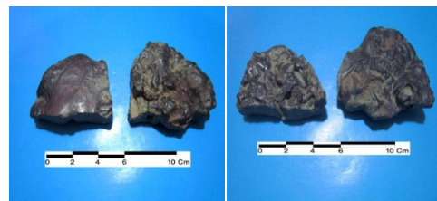
Fig8. Right: Upper Surface of the Flat Slags with Flow Wrinkles; Left: Lower Surface of the Specimen with Flat Morphology at the Left in Contrast to Irregular Morphology of Upper Surface at the Right.
