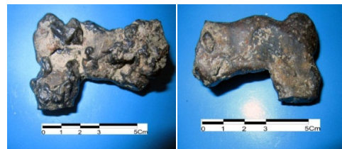
Fig10. Right: Upper Surface of the Specimen with Bulging, Reform Morphology that Reflects Plastic Deformations of the Melt during its Freezing Process; Left: Lower Surface of the Specimen Characterized by Relatively Irregular Morphology, Concentration of Secondary White Minerals Around
